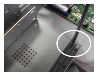
Figure 3: Remove screws from the bracket
